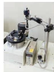
Atomic force microscope (AFM) with molecular-level resolution under controlled environment used to clarify the mechanism of radioactive contaminant removal
