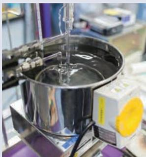
CO oxidation reaction experiment: Glass tube is filled with sample catalyst and immersed in a constant temperature bath.
