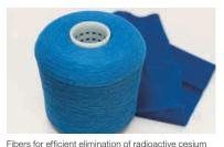
Hibers for efficient elimination of radioactive cesium from contaminated wastewater from the seeded log decontamination instrument and combustion gas removal instrument
